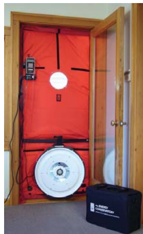
Testing Building Air Tightness with a Minneapolis Blower Door
